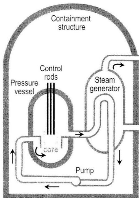
Figure 1. A schematic diagram of nuclear reactor.
