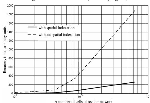
Fig. 2. Comparison of numerical efficiency of geofield recovery algorithms
