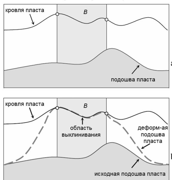
**Fig. 1.** The example of refining oil stratum configuration: a) before editing and b) after
